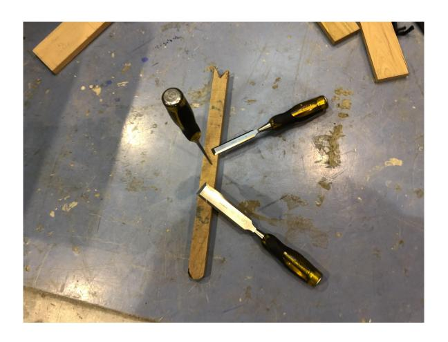
The chisel is one of the first indispensable tools for carpenter! It's used to make notches!
